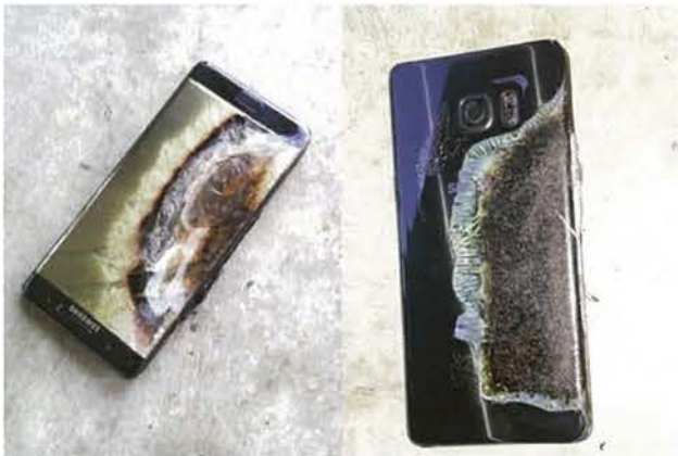
SAMSUNG'S NEWEST GALAXY DEVICE, THE NOTE 7, WAS RECALLED FOR DEFECTIVE BATTERIES AND CHARGING SYSTEMS THAT CAUSED THEM TO OATCH FIRE.
