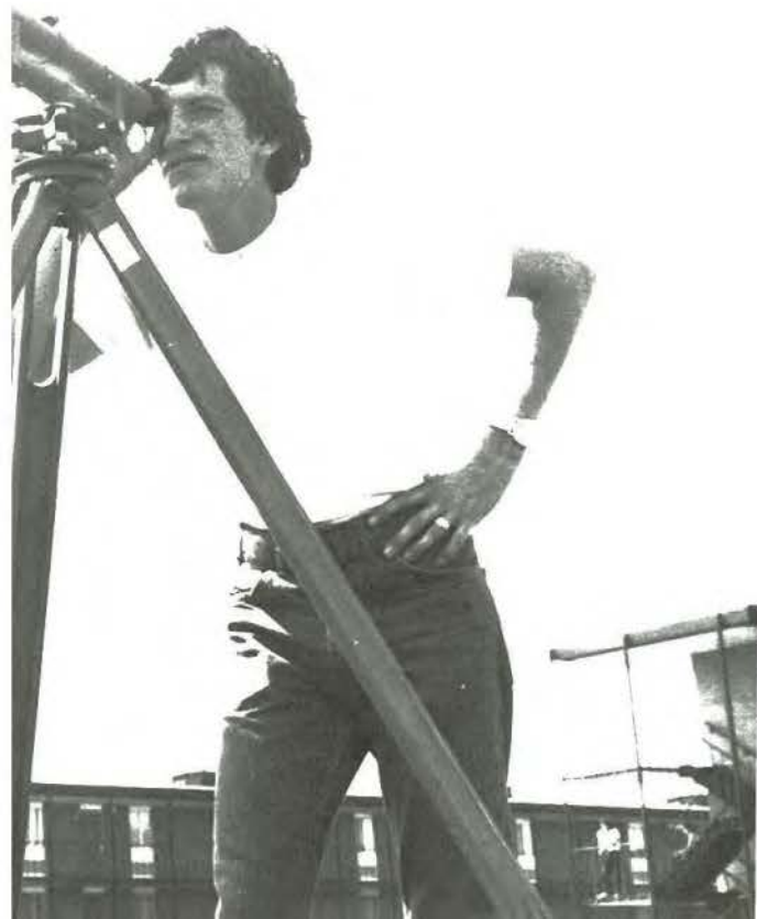
Ron Pollert and Wayman Spangler shoot elevations for a level circuit as an in-the-field application of principles and techniques learned in Surveying class. Student gains are of prime importance as this newly reorganized division provides opportunities for professional development, personal development and career exploration through the diversity of classes offered.
